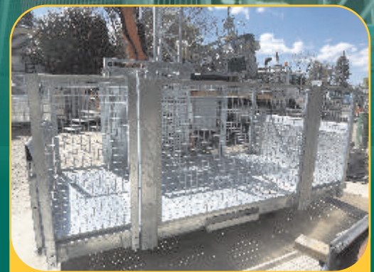
Full 3.2m long platform for sheets of gyprock / plywood.
